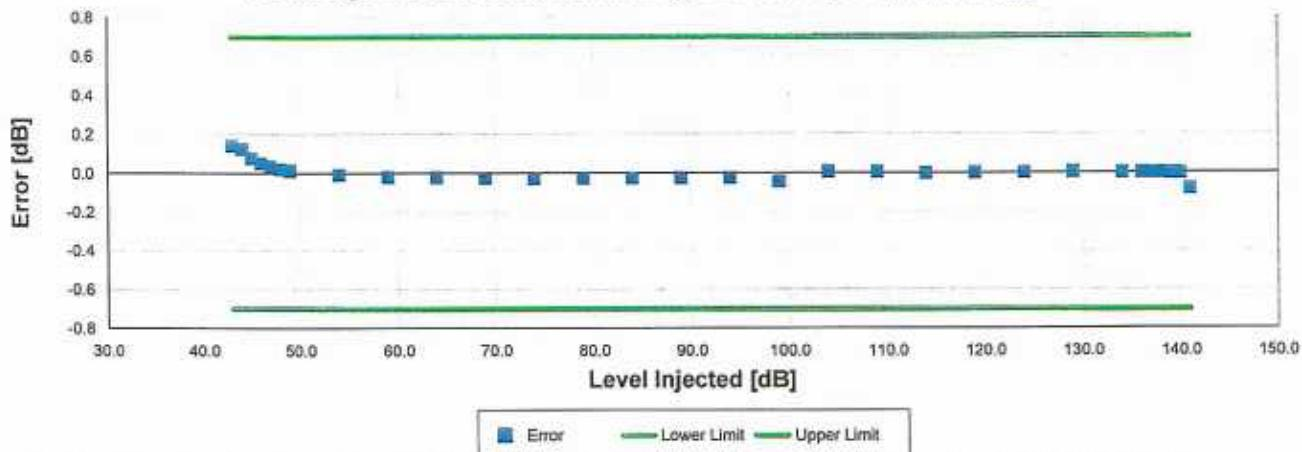
Broadband level linearity performed according to IEC 61672-3:2013 16 and ANSI S1.4-2014 Part 3: 16 for compliance to IEC 61672-1:2013 5.6, IEC 60804:2000 6.2, IEC 61252:2002 8, ANSI S1.4 (R2006) 6.9, ANSI S1.4-2014 Part 1: 5.6, ANSI S1.43 (R2007) 6.2
