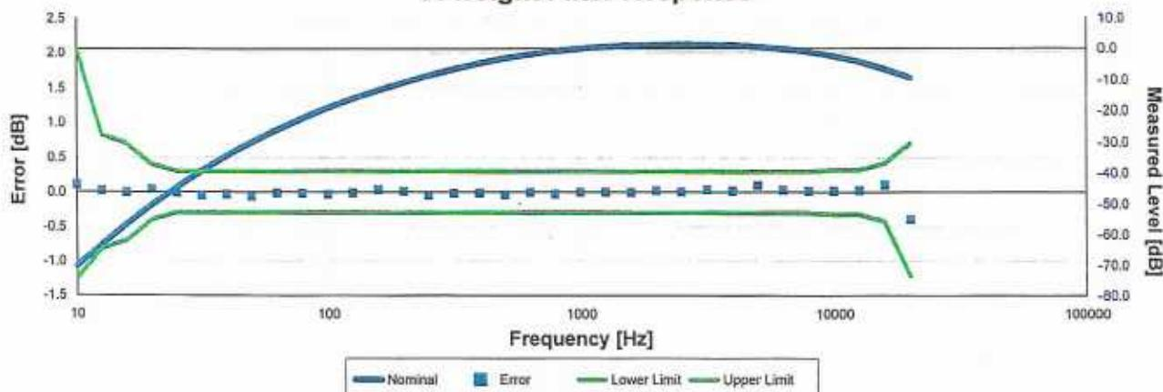
Electrical signal test of frequency weighting performed according to IEC 61672-3:2013 13 and ANSI S1.4-2014 Part 3: 13 for compliance to IEC 61672-1:2013 5.5; IEC 60651:2001 6.1 and 9.2.2; IEC 60804:2000 5; ANSI S1.4:1983 (R2008) 5.1 and 8.2.1; ANSI S1.4-2014 Part 1: 5.5
