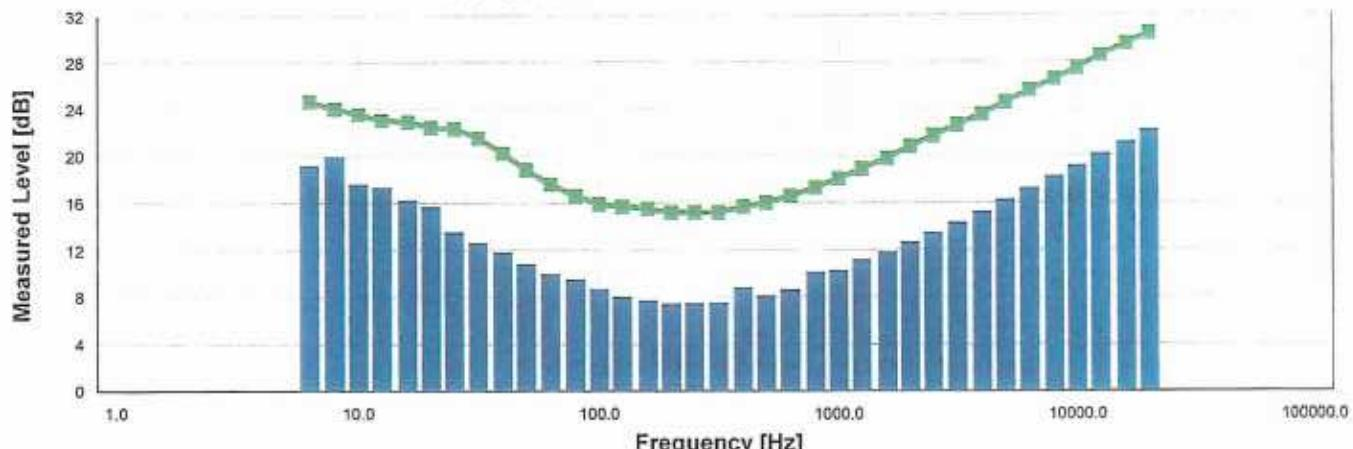
The SLM is set to low range. 1/3-Octave self-generated noise measured according to IEC 61672-3:2013 11.2 and ANSI S1.4-2014 Part 3: 11.2
