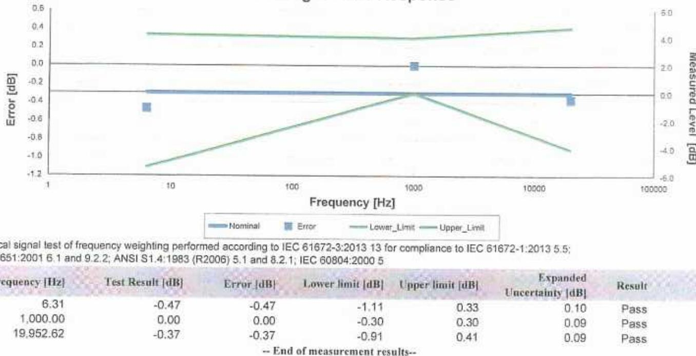
Electrical signal test of frequency weighting performed according to IEC 61672-3:2013 13 for compliance to IEC 61672-1:2013 5.5; IEC 60651:2001 6.1 and 9.2.2; ANSI S1.4:1983 (R2006) 5.1 and 8.2.1; IEC 60804:2000 5
