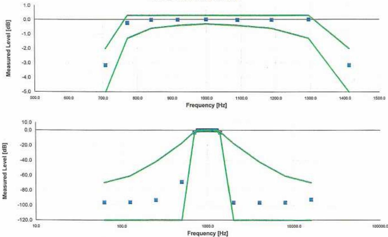
Filter shape measured according to IEC 61260:2001 and ANSI S1.11:2004
