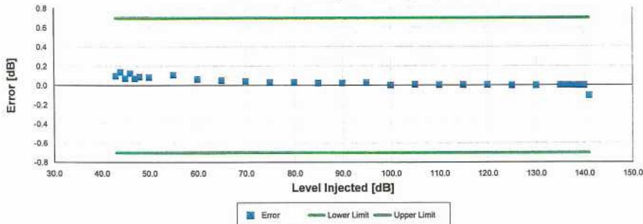
1/3 octave level linearity at normal range performed according to IEC 61260:2001 4.6, ANSI S.11 (R2009) 4.6
