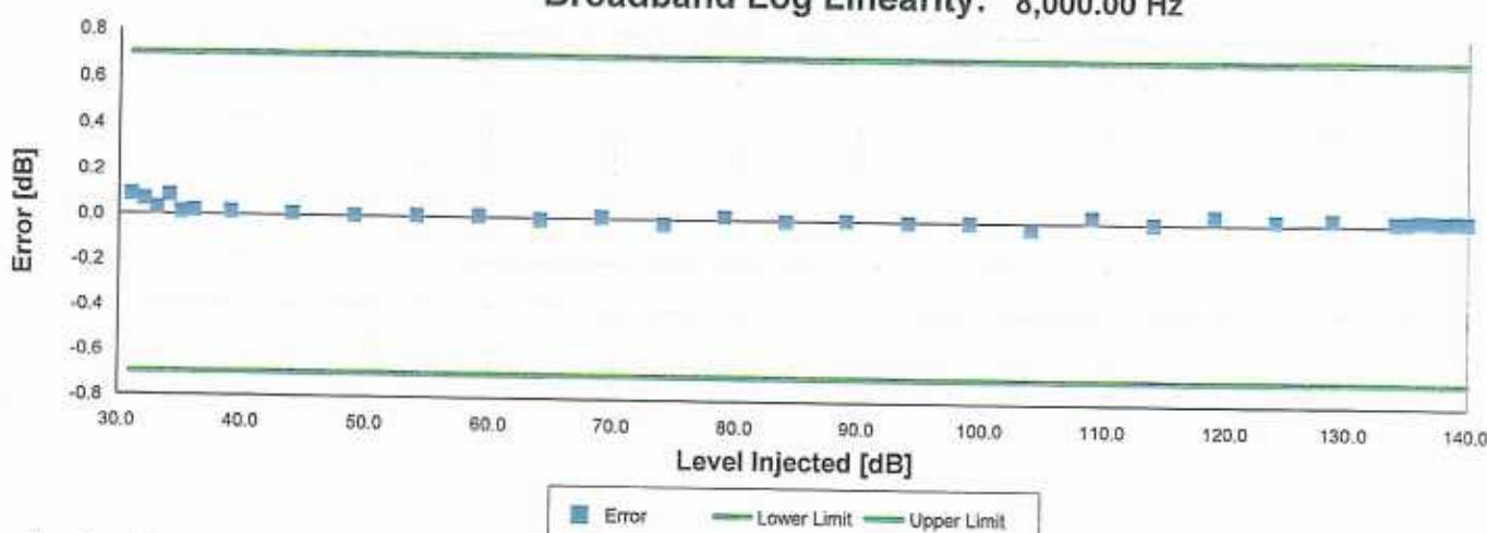
Broadband level linearity with 0 dB gain performed according to IEC 61672-3:2013 16 for compliance to IEC 61672-1:2013 5.6, IEC 60604:2000 6.2, IEC 61252:2002 8, ANSI S1.4 (R2006) 6.9, ANSI S1.43 (R2007) 6.2
