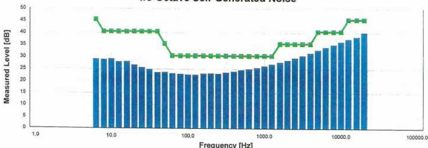
The SLM is set to low range and 0dB gain. 1/3-Octave self-generated noise measured according to IEC 61672-3:2013 11.2
