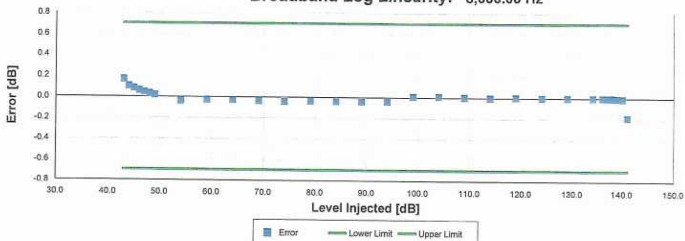
Broadband level linearity with 0 dB gain performed according to IEC 61672-3:2013 16 for compliance to IEC 61672-1:2013 5.6, IEC 60804:2000 6.2, IEC 61252:2002 8, ANSI S1.4 (R2006) 6.9, ANSI S1.43 (R2007) 6.2
