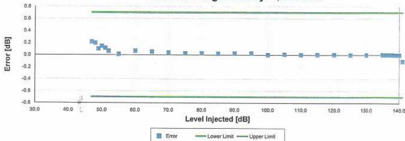
1/1 octave level linearity at normal range performed according to IEC 61260:2001 4.6, ANSI S.11 (R2009) 4.6
