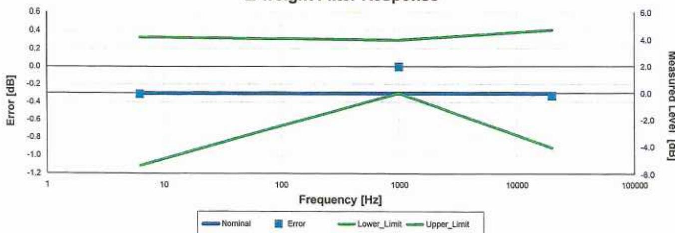
Electrical signal test of frequency weighting performed according to IEC 61672-3:2013 13 for compliance to IEC 61672-1:2013 5.5; IEC 60651:2001 6.1 and 9.2.2; ANSI S1.4:1983 (R2006) 5.1 and 8.2.1; IEC 60804:2000 5
