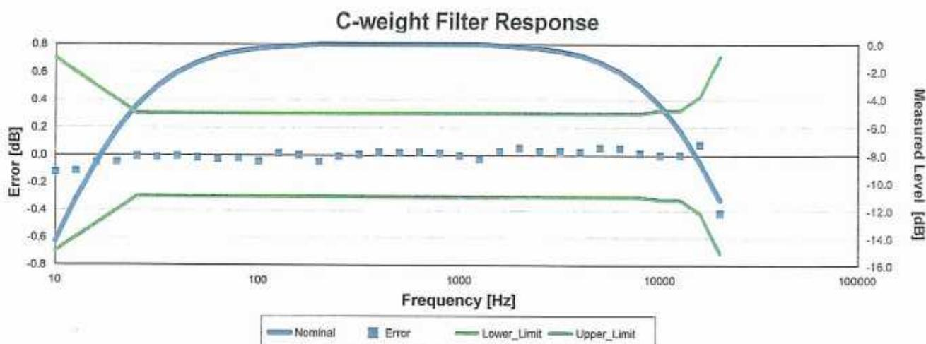
Electrical signal test of frequency weighting performed according to IEC 61672-3:2013 13 and ANSI S1.4-2014 Part 3: 13 for compliance to IEC 61672-1:2013 5.5; IEC 60651:2001 6.1 and 9.2.2; IEC 60804:2000 5; ANSI S1.4:1983 (R2006) 5.1 and 8.2.1; ANSI S1.4-2014 Part 1: 5.5
