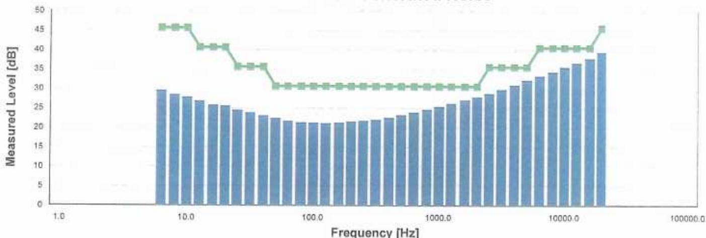
The SLM is set to low range and 0dB gain. 1/3-Octave self-generated noise measured according to IEC 61672-3:2013 11.2.
