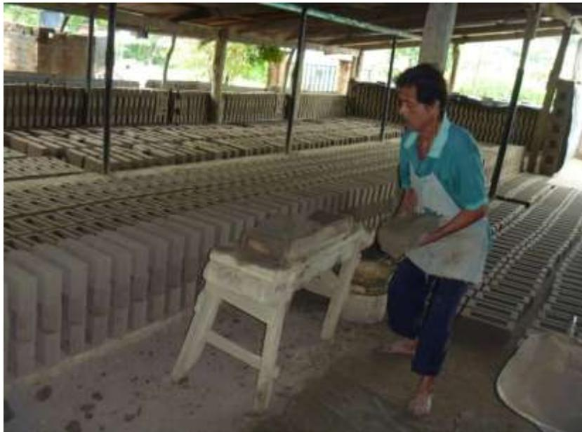
**Fig.10** Moldeo de ladrillo
