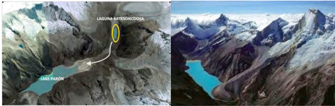
Left: The path taken by the 1951 outburst floods from Artesoncocha into Lake Parón. Google Earth imagery is from 2012. Right: Lake Parón showing the moraine descending from Huandoy that blocked the valley and created the lake. Photo: César Portocarrero
