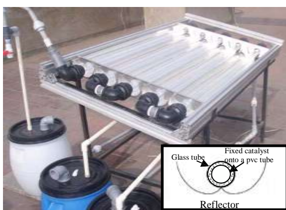
Figure 1: a) Scheme of the laboratory reactor. The inset shows a cross section of the irradiation systems.
